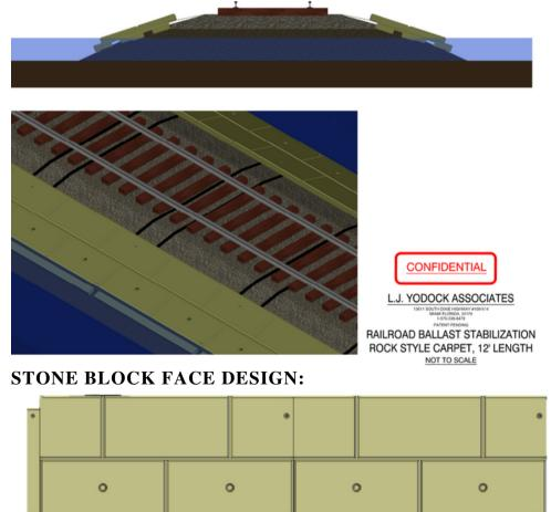
The Rock Carpet product would be utilized to handle a reoccurring failure (erosion) spaulding of an original wall or railroad track infrastructure. The rock carpet could provide additional structural integrity to installation trouble spots.
